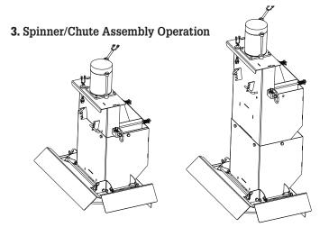
Attach chute to hopper assembly by inserting tabs into slots in chute motor plate. Then secure chute by engaging spring latches in respective holes. Chute heights can be adjusted by attaching lower chute weldment to the upper one using upper or lower set of holes. Two sets of holes are located on the bottom of upper chute weldment and under internal baffles selectors.
