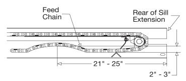
To check the tension, measure in 21"-25" from the rear edge of the gear box mount. Push up on the chain with your hand. The conveyor chain should lift up 2"-3" off the conveyor chain guide or cross angles.
