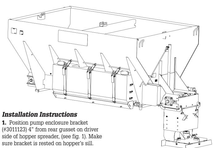
**2.** Weld pump enclosure bracket (#3011123) in place as shown in fig.1.
