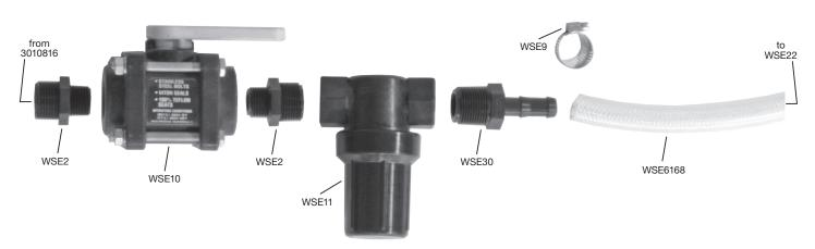
Fig. 8 Filter/Valve Assembly
