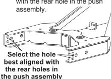
If your configuration has a locking plate (T-Frame Locking Kit, PN 29735), rotate the locking plate as shown to match the hole in the rear of the T-frame.
