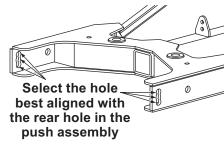
Rotate the locking plate to match the selected hole.
