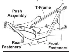
to the T-frame. Loosen the front fasteners, and allow the blade to find a level position.
