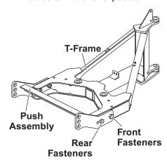
5. Select the hole in the rear of the T-frame that is best aligned with the rear hole in the push assembly.
