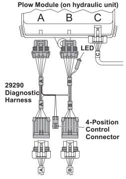
Connect the diagnostic harness connectors A and B to the matching ports on the Plow Module (A to A and B to B).
