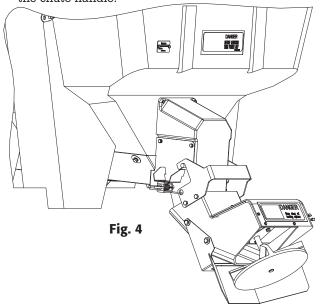
**B.** Rotate the Chute into operating position and lock using two spring latches.
