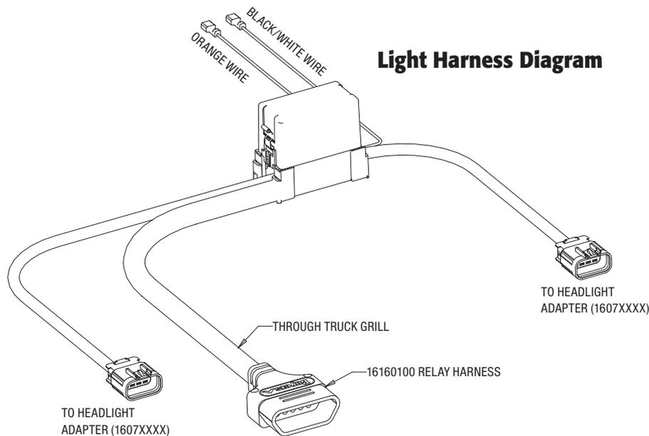
1. Route the RELAY HARNESS through the grill (drivers side preferably) and place the RELAY MODULE close to either the drivers or passenger side headlight (whichever is convenient).
