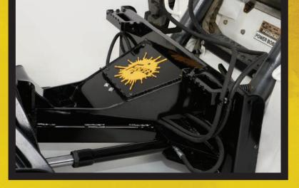
A universal skid-steer loader mounting plate makes hook-up fast and easy. The skid-steer's standard auxiliary hydraulic system provides the power to angle the blade.
