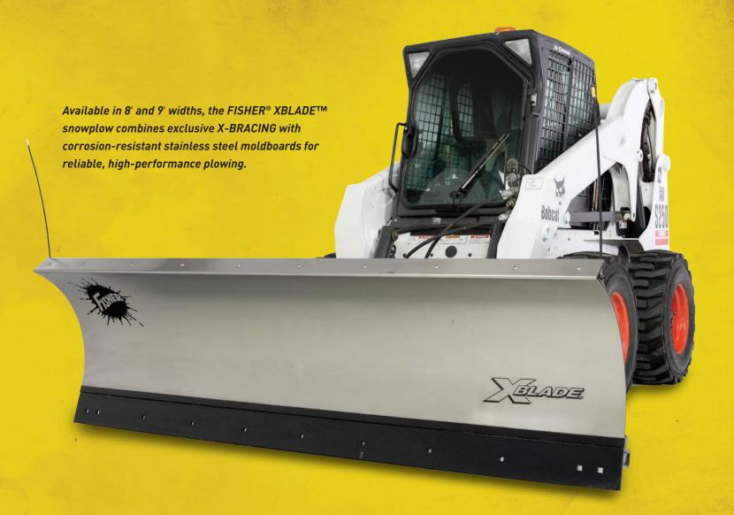
The proven FISHER XBLADE and HD Series snowplows are available with a universal skid-steer loader mounting plate for fast and easy hook-up. The skid-steer's standard auxiliary hydraulic system provides the power to angle the blade. With Fisher Engineering's proven trip-edge design, only the edge trips back when striking an obstacle, leaving the blade upright and plowed snow in front of the blade.
