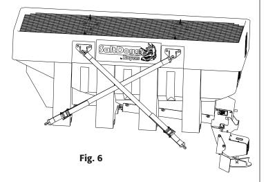
Verify with the vehicle's manufacturer that the factory installed anchor points are designed for tie-down such load. Inspect straps and hardware after each time spreader is loaded. Tighten straps and hardware if necessary.
