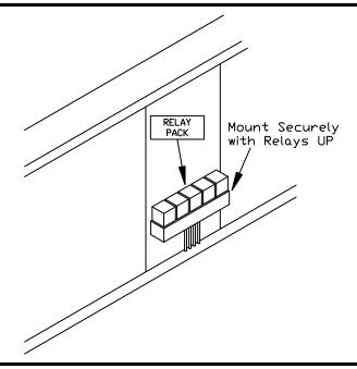
Figure 21. Relay Mounting.
