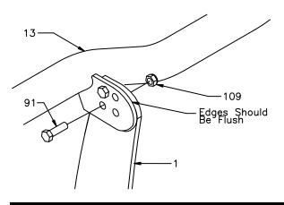
Figure 6. Light Bar Assembly. (Standard)
