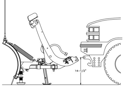
Figure 39. Recommended Push Beam Height- Sport Duty
