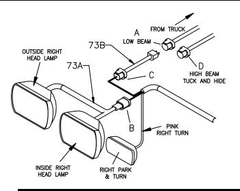
Figure 25. Dual Headlight Adapter ConnectionsG10151
