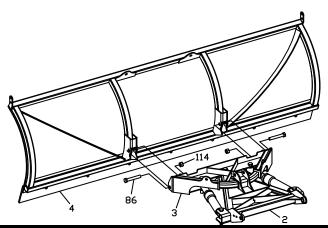
Figure 2. Push Frame Attachment
