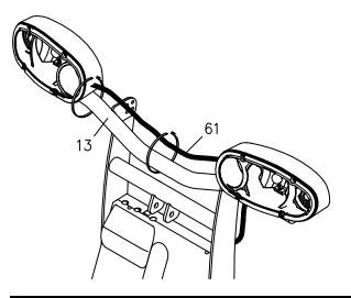
Figure 9. Securing Wiring Harness
