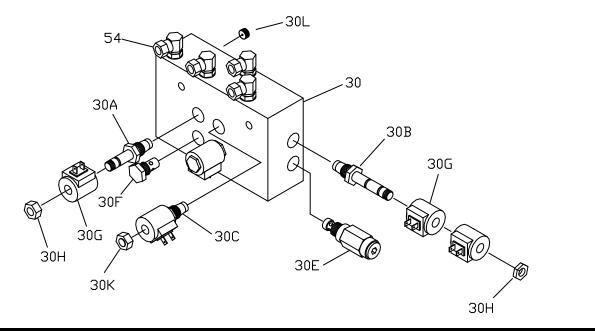
Figure 34. Straight Blade (Sport) Manifold with SmartHitch2<sup>™</sup> Parts Diagram
