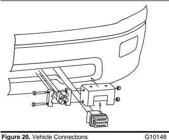
29. Mount the Black 13 Pin Control Harness Connector to the lower area of the bumper using **MSC03813** Control Harness Mounting Bracket.
