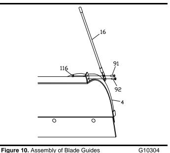
Figure 10. Assembly of Blade Guides
