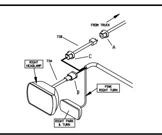
Figure 24. Single Headlight Adapter ConnectionsG10149
