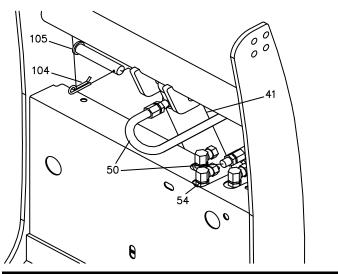
Figure 12. Installing SmartHitch2<sup>™</sup> Hose
