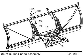
Figure 3. Trip Spring Assembly
