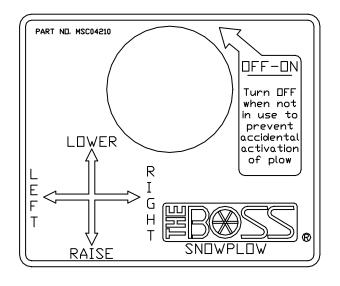
Figure 35. Straight Blade Control Operation G10154
