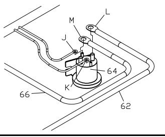
Figure 18. Solenoid Connections.
