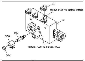
**Figure 11.** SmartHitch2<sup>™</sup> Valve Installation G10130
