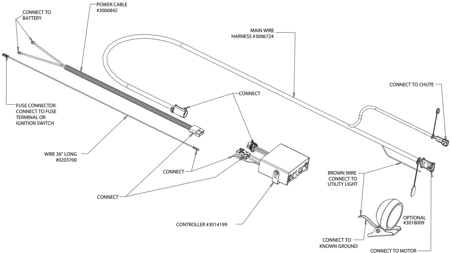
**G.** Make sure that the Controller is OFF. Connect the small female terminal on the blue wire to the controller Ignition (single red) wire. Connect the blue wire to an accessory wire, terminal or fuse that is controlled by the vehicle's ignition switch located in the fuse panel inside the truck cab. **Do not connect blue wire to high amperage fuse or terminal.**
