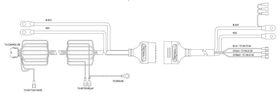
The portion on the left is the TRUCK HARNESS, and is routed between the bumper (plow interface) and under the dashboard (for the controller and ignition power connections). The portion on the right is the PLOW HARNESS and comes pre-assembled to the plow. It is used during assembly for the initial plow setup and testing.
