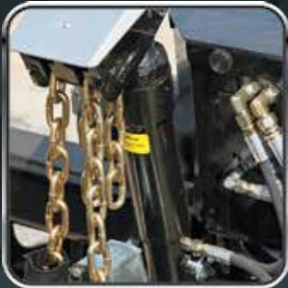
5 Lift Arm - 35° travel provides exceptional snow stacking. Heavy-Duty 2" x 6" lift cylinder.
