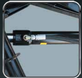
8 Double Angle Cylinders - for REAL backdragging, standard
