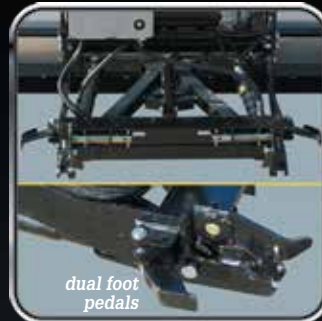
3 Quick Attach/Detach Mounting - easy to use over center linkage operated locking pins with foot pedals
