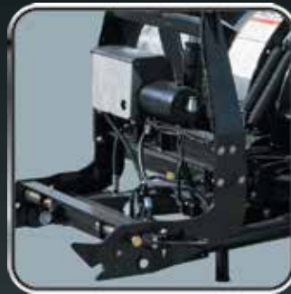
7 Contoured Lift Frame - for greater ground clearance
