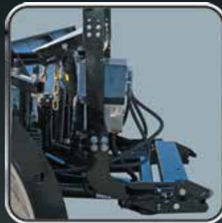
7 Contoured Lift Frame - for greater ground clearance
