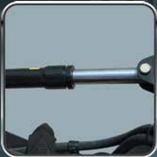
9 1 1/2" x 12" Angle Cylinders - delivers greater angling force than standard cylinders
