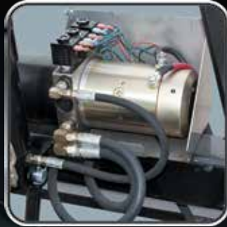
2 Power Unit / Hydraulics full size SAE std. cartridge valves, oversized 3/8" rubber hoses, integral valve manifold
