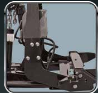
8 Contoured Lift Frame - for greater ground clearance
