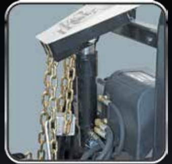
4 Lift Arm - 35° travel provides exceptional snow stacking. Heavy-Duty 2" x 6" lift cylinder.
