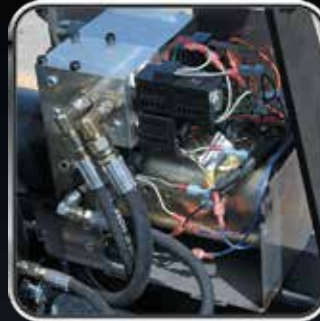
3 Power Unit / Hydraulics full size SAE std. cartridge valves, oversized 3/8" rubber hoses, integral valve manifold
