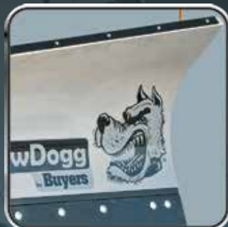
10 Moldboard - tough stainless steel corrosion free moldboard
