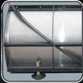
1 ¼" Laser Cut Steel Ribs w/ 2" Cross Tube & HD Channel spreads loads across components not connection points
