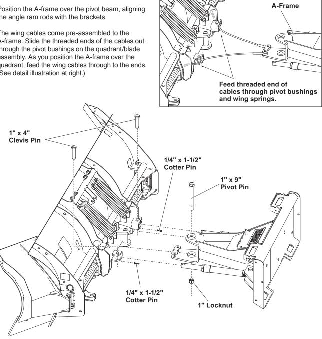
5. Assemble a 3/4" hex nut and 3/4" jam nut loosely onto the threaded end of each cable. Thread the nuts on just flush with the end of the cable.
