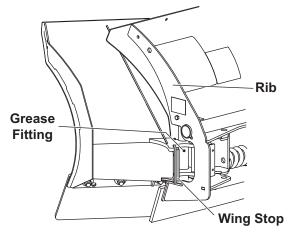
2. If there is a gap between the wing stop and the rib, skip to Step 3.
