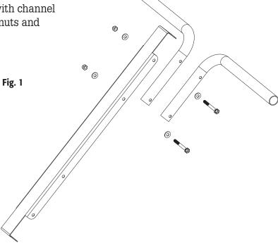
**2.** Assemble lower support arms (3016745 and 3016744) in channel as shown using supplied  $^{1}$ 4-20 bolts, nuts and washers. Insert control rod (3016748) and handle (3016760). Do not tighten set screw at this time. See fig 2.
