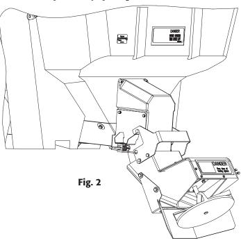
Then rotate the Chute into operating position and lock using two spring latches.
