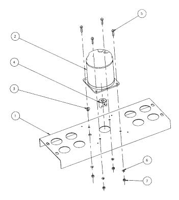
Fig. 3 Motor Base Assembly
