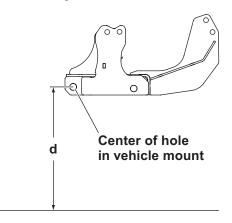
2. Use the following chart to determine the proper A-frame hole position.
