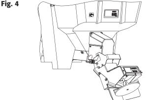
**B.** Rotate the chute into operating position and lock using the two spring latches.
