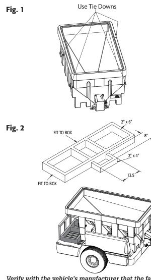
Verify with the vehicle's manufacturer that the factory installed anchor points are designed for tie-down such load. Inspect straps and hardware after each time spreader is loaded. Tighten straps and hardware if necessary.
