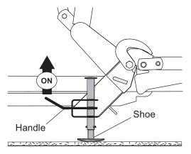
2. Pull and hold the lock pin out; then rotate the handle UP and release the lock pin. It must lock into the UPPER hole. The stand hook must grip the receiver pin.
