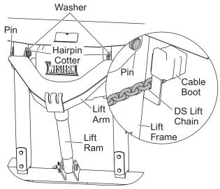
6. Unhook the driver-side lift chain from the lift frame and hook the marked chain link onto the lift arm.
