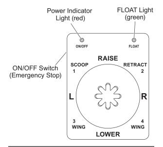
NOTE: If a control function times out before the desired blade movement is complete, release the lever to the center position, then move it back into the desired function.
