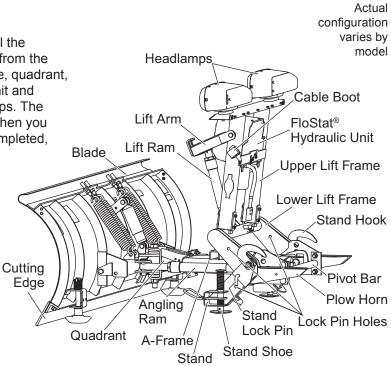
The snowplow shall be installed according to instructions supplied. WESTERN<sup>®</sup> outlets are trained to provide this service and other services for this snowplow.
