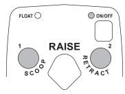
The two round buttons located to the left and right of the RAISE button move both wings at the same time into the blade positions described in the following table.
