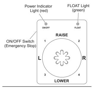
NOTE: If a control function times out before the desired blade movement is complete, release the lever to the center position, then move it back into the desired function.
