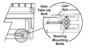
3. Loosen the jam nut on one of the take-up bolts, then tighten (clockwise) the take-up bolt one full revolution. Repeat evenly on the other side.
