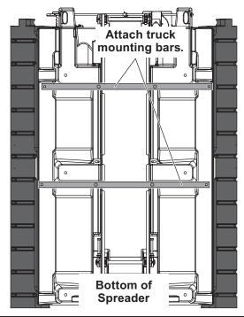
4. The spreader can be moved into the truck bed either by lifting the spreader by the four molded-in handles located on the corner legs or by sliding the spreader into the truck bed from the ground.
