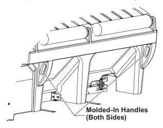
To lift the spreader into the truck bed from the ground, stand the spreader up on the feet at the rear of the spreader on top of two spacers at least 2" off the ground. The chute must be removed.
