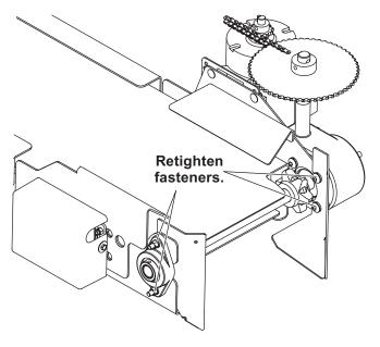
c. Tighten all of the fasteners according to the torque chart.
