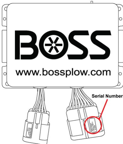
Figure 2. Serial Number and REV Level Location G13933
