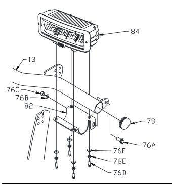
Figure 1. Headlight Mounting Assembly
