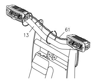
Figure 3. Secure Wiring Harness
