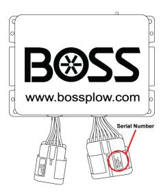
Figure 2. Serial Number and REV Level Location
