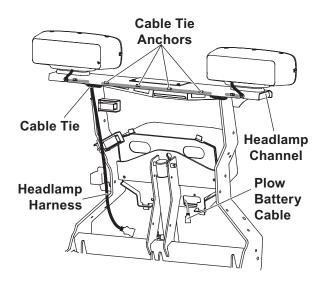
5. Cable tie the harnesses and battery cable to the headgear as shown in illustration.
