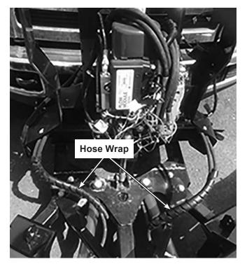
6. Install the provided hose wrap as shown to prevent the hoses from chafing and premature wear.
