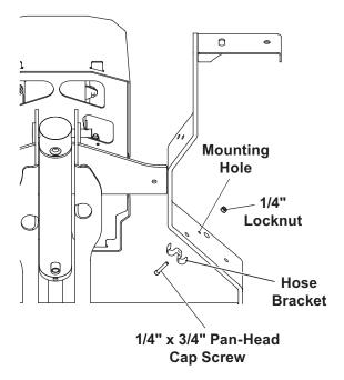
4. Adjust the position of the hoses so that they will have slack when the lift ram is fully extended and will not be stretched on either side of the hose bracket.
