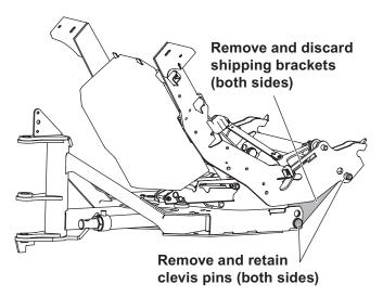
Remove and discard the shipping brackets and the two cap screws and locknuts from the lift cylinder.
