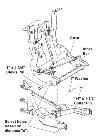
3. Fold the headgear forward and pin the lift cylinder to the T-frame using a 5/8" x 4-1/4" clevis pin and 1-1/2" x 5/32" cotter pin from the parts bag.
