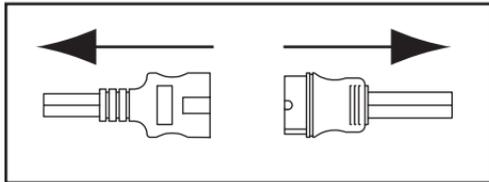
**NOTE:** After each use of the snowplow, reapply dielectric grease to the electrical plugs to maintain the protective coating on the terminals.
