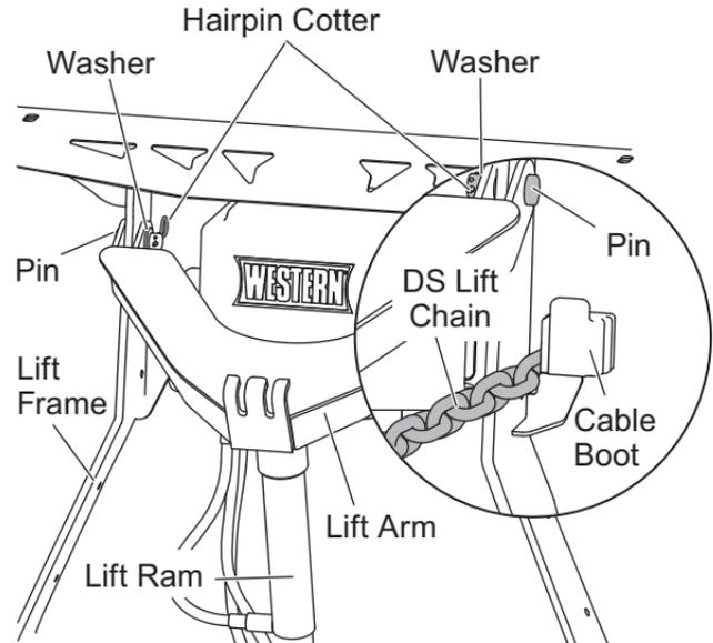
6. Unhook the driver-side lift chain from the lift frame and hook the marked chain link onto the lift arm.
