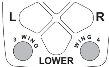
The two round buttons located to the left and right of the LOWER button move either wing independently of the other as described in the following table.
