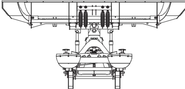
2. Standing behind the blade, install a 3/4" x 9" clevis pin down through the holes in the back of the blade assembly, as shown.
