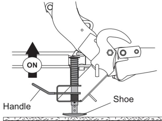
2. Pull and hold the lock pin out; then rotate the handle UP and release the lock pin. It must lock into the UPPER hole. The stand hook must grip the receiver pin.
