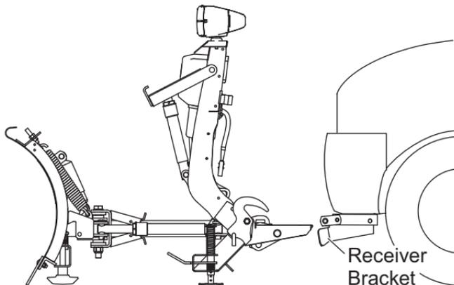
Two removable receiver brackets are attached to the mount using pins and hairpin cotters. The receiver brackets are easily removed to provide more road clearance during the non-plowing months of the year.
