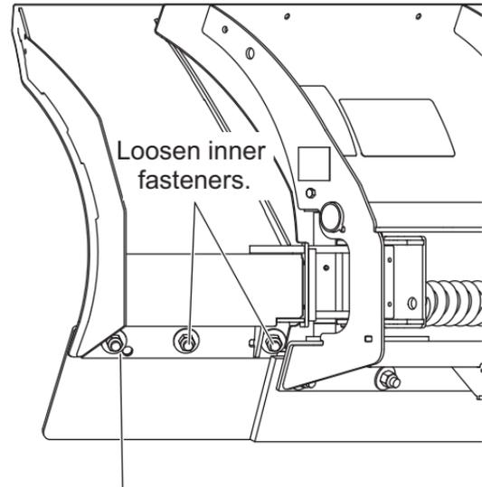
Remove outer fastener and reinstall in lower hole.
