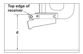
2. Use distance "d" from Step 1 and the following chart to determine the proper pivot plate hole position.
