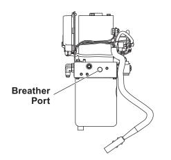
6. Install the 90° elbow into the port, pointing up. Install the breather into the elbow.
