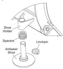
Standard shoe kit shown. An optional shoe kit, available for the HT Series $^{\text{TM}}$  and SD series blades, has a bolt-on shoe holder.
