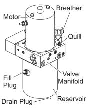
The HT Series™ hydraulic unit has blade scrape lock circuitry built into it. This feature resists the tendency a snowplow has to "float up" as larger amounts of snow build up in front of it while plowing deep snow, or stacking snow into piles. This feature is activated when the blade is in FLOAT, and is factory set. See your sales outlet for adjustment. The HT Series blade is raised in approximately 4 seconds and angled side to side in approximately 3 seconds.
