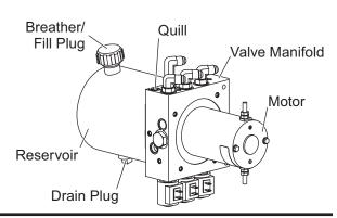
The XtremeV<sup>™</sup> blade is raised in approximately 2 seconds and angled side to side in approximately 2 seconds.
