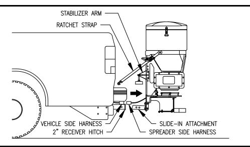
Figure 6. Slide-In Attachment Removal Procedure
