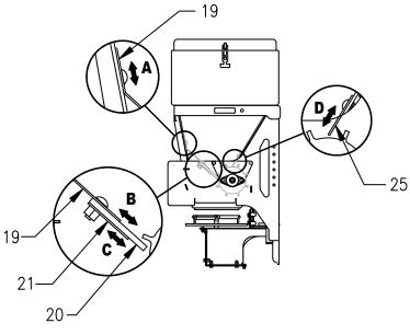
Figure 20. Vibration Tray Adjustment G10609
