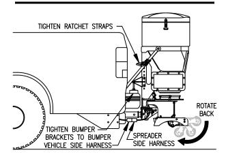
Figure 11. Stabilizer Arm Adjustment G10601
