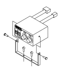
Figure 17. In-Cab Controller Installation Procedure
