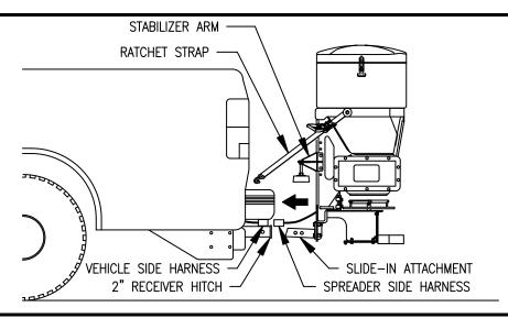
Figure 5. Slide-In Attachment Mounting Procedure
