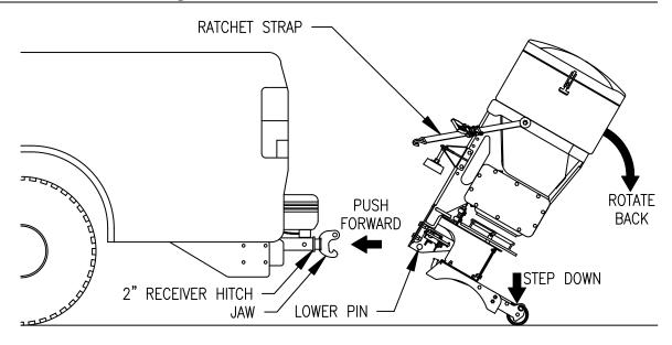
Figure 10. RT3 Attachment Mounting Procedure
