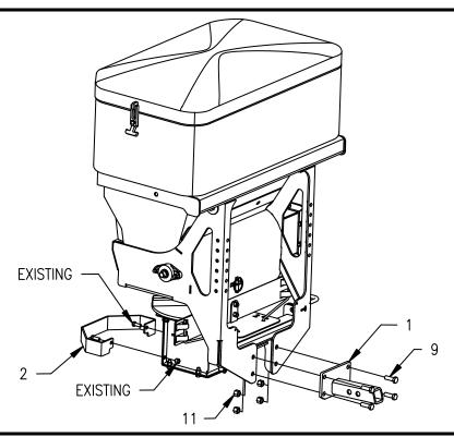
Figure 4. Slide-In Attachment Installation Procedure
