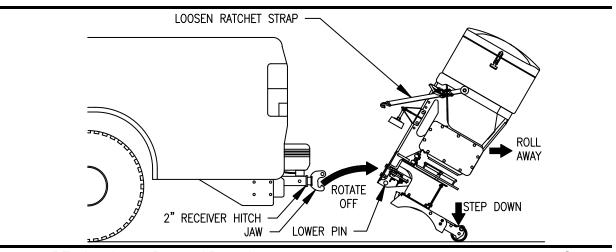
Figure 13. RT3 Attachment Removal Procedure
