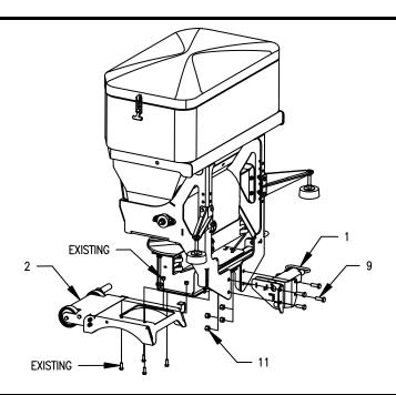
Figure 7. RT3 Attachment Installation Procedure
