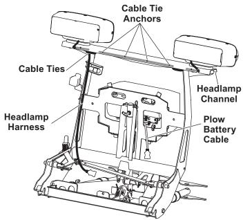
5. Cable tie the harness to the headgear as shown in illustration.
