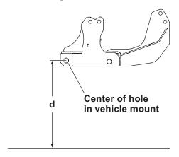
2. Use distance "d" from Step 1 and the following chart to determine the proper A-frame hole position.
