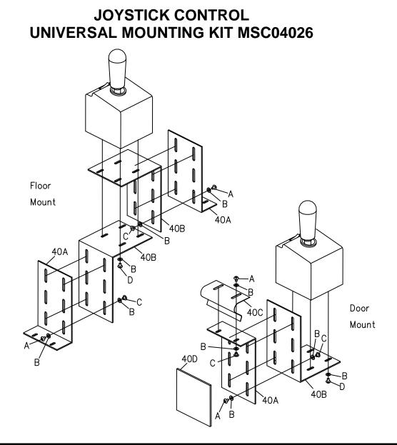
Figure 39. Joystick Control Universal Mounting Kit Components
