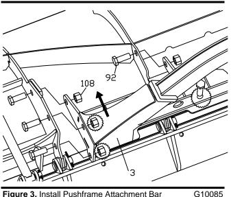
Figure 3. Install Pushframe Attachment Bar
