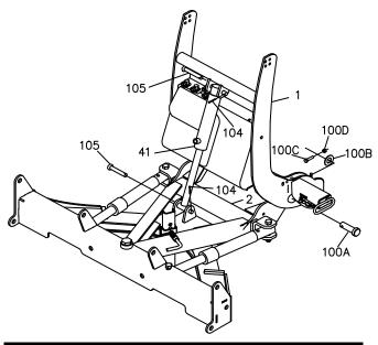
Figure 6. Lift Cylinder Installation
