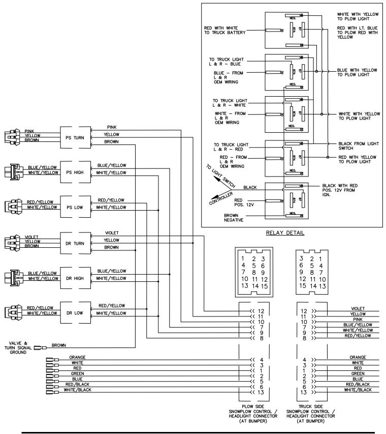
Figure 29. Electrical System Wiring Schematic (Plow Side)
