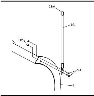
Figure 13. Assembly of Blade Guides.
