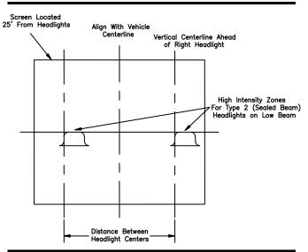
Figure 30. Headlight Aiming Procedure
