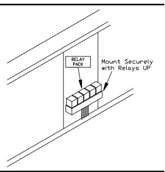
Figure 24. Relay Mounting.
