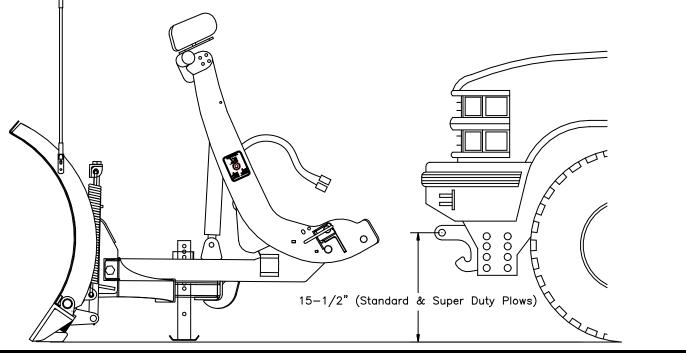
Figure 42. Recommended Pushbeam Height
