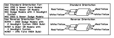
Figure 25. Vehicle Option Connector
