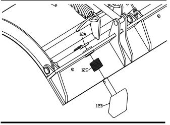
Figure 2. Install Shoe Assembly
