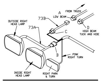
Figure 28. Dual Headlight Adapter Connections G10151
