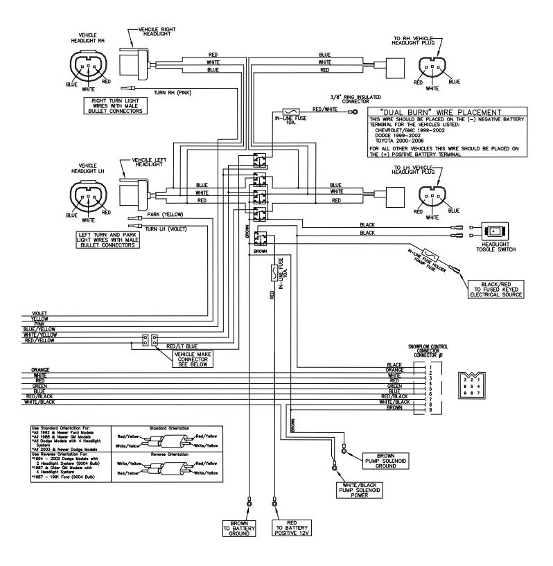
Electrical System Wiring Diagram
