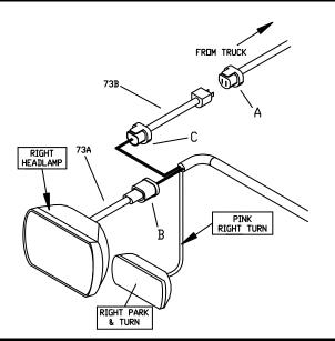
Figure 27. Single Headlight Adapter Connections G10149
