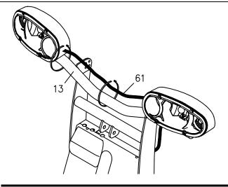
Figure 12. Securing Wiring Harness
