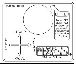
Figure 38. Straight Blade Control Operation G10154
