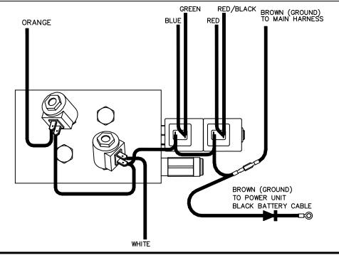
Figure 32. HYD07090 Standard Duty Manifold Wiring Diagram
