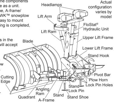
There is no need to unhook the chains or the hydraulic hoses. When the lift frame is pinned to the stands and locked in place (see blade label or snowplow removal section of this manual), the complete UltraMount<sup>®</sup> snowplow can easily be moved around on most hard surfaces.
