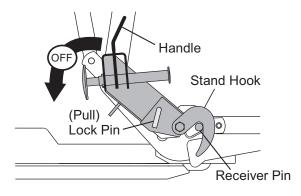
Push down top of shoe; shoe will be on the ground. Repeat Steps 2 and 3 on other side of snowplow (not required for HTS<sup>™</sup> blades). Back vehicle away.
