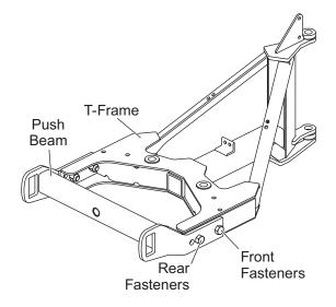
6. Select the hole in the rear of the T-frame that is best aligned with the rear hole in the push beam and reinstall the rear fasteners. Tighten all four fasteners to 250 ft-lb.
