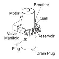
The HTS<sup>™</sup> hydraulic unit has blade scrape lock circuitry built into it. This feature resists the tendency a snowplow has to "float up" as
