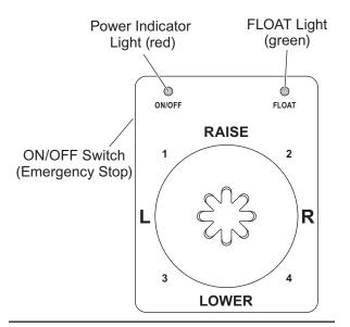
NOTE: If control function times out before desired blade movement is complete, release the lever to the center position, then move back into the desired function.
