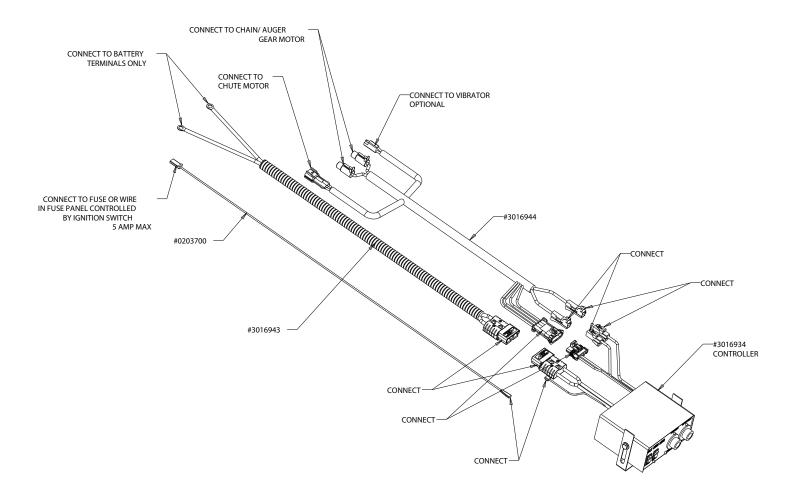
Thoroughly clean battery terminals. Make sure battery terminals have no tarnish or corrosion. DO NOT CONNECT WIRE HARNESS TO DAMAGED OR CORRODED TERMINALS!
