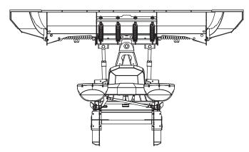
Fully angle the blade to one side. Lower the blade and turn the plow control and vehicle ignition OFF.
