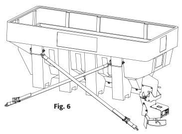
Verify with the vehicle's manufacturer that the factory installed anchor points are designed for tie-down such load. Inspect straps and hardware after each time spreader is loaded. Tighten straps and hardware if necessary.
