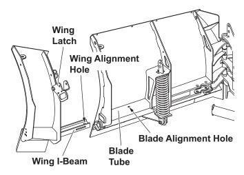
4. Insert a 3/8" pin through the blade alignment hole and wing alignment hole. Secure with a hairpin cotter.
