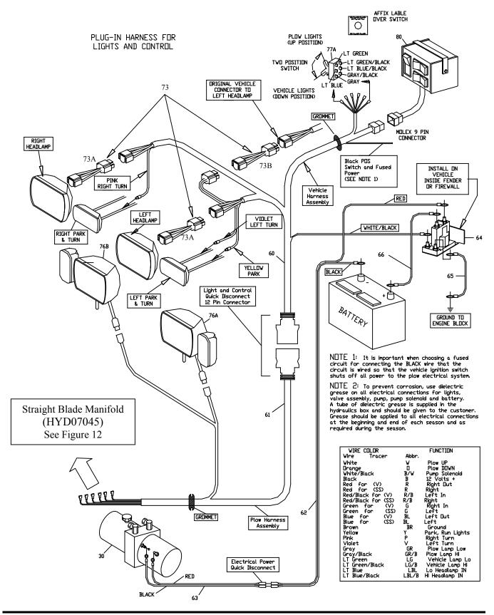
Figure 7. RT3 Wiring Diagram
