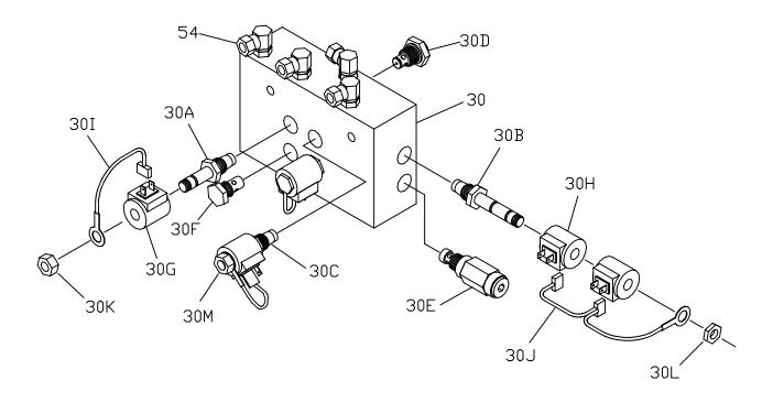
Figure 9. Straight Blade Manifold with SmartHitch™ Parts Diagram
