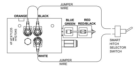
Figure 4. RT3 Straight Blade with SmartHitch™ Manifold
