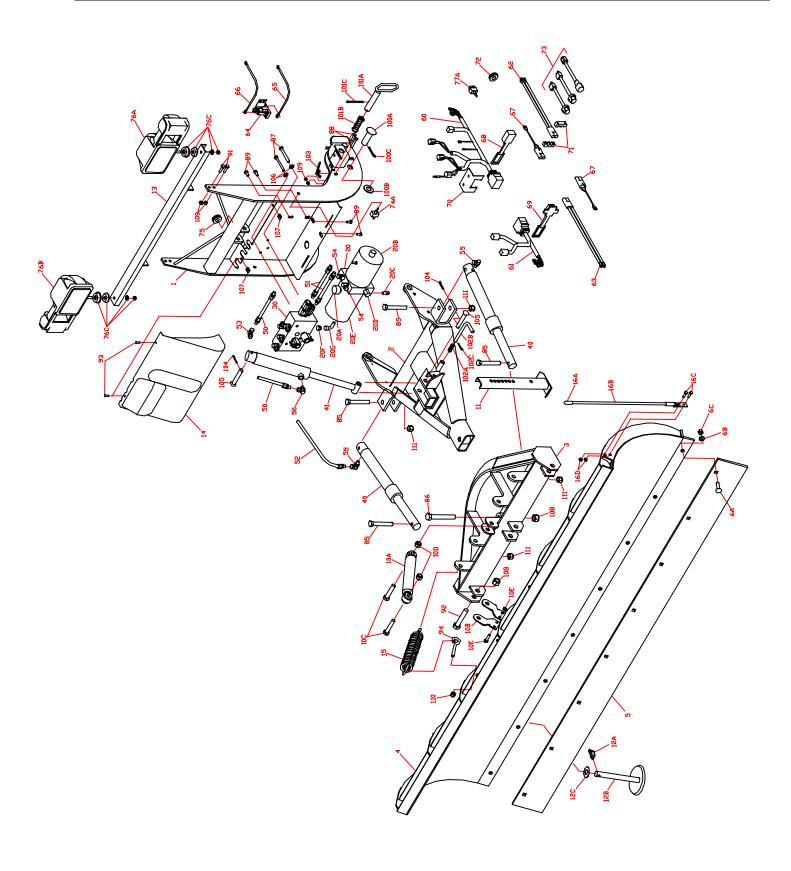
Figure 10. RT3 Straight Blade Assembly Drawing
