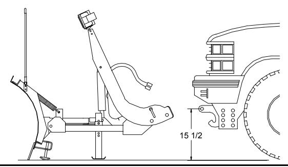
Figure 11. RT3 Recommended Pushbeam Height
