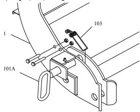
Cap Screw (88) and **HDW01720** Self-Locking Nut (109). Align the top of the spring with the center of the spring pin hole, then tighten. For the 10' Super Duty, use **MSC07673** SmartHitch™ Torsion Springs (103) and **HDW05573** Hex Head Cap Screw (88).
