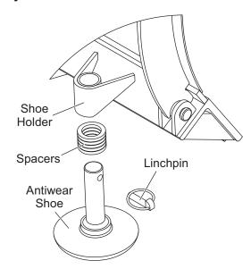
Standard shoe kit shown. An optional shoe kit, available for the HT Series<sup>™</sup> and SD series blades, has a bolt-on shoe holder.
