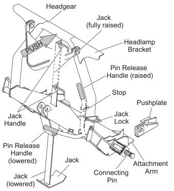
HT Series™ (Dual Jack Legs): Pull and hold jack lock out. Lower jack until it contacts the ground. Release jack lock. Verify that jack is locked by trying to lift jack. Repeat on opposite side. For illustration, see p. 87.
