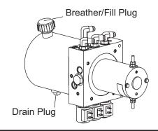
6. **HT Series™ Blades:** Fill the reservoir to within 2-1/2" from the top of the fill hole and replace the fill plug.
