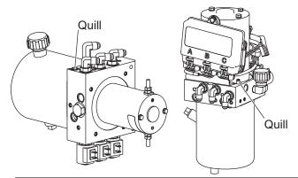
The quill in the valve manifold adjusts the blade drop speed.
