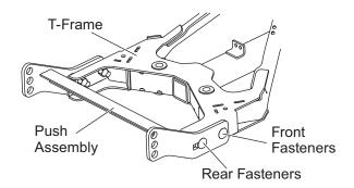
4. Select the hole in the rear of the T-frame that is best aligned with the rear hole in the push assembly and reinstall the rear fasteners. Tighten all four fasteners to 250 ft-lb.
