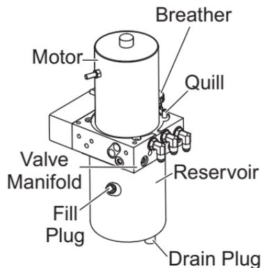
The HTS™ hydraulic unit has blade scrape lock circuitry built into it. This feature resists the tendency a snowplow has to "float up" as
