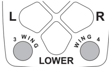
The two round buttons located to the left and right of the LOWER button move either wing independently of the other as described in the following table.
