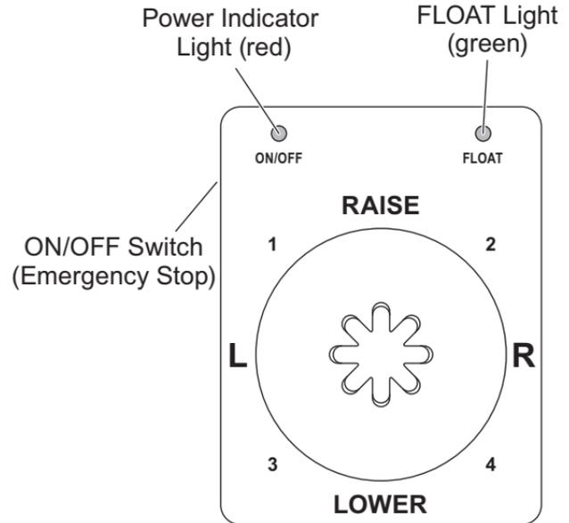
**NOTE:** If control function times out before desired blade movement is complete, release the lever to the center position, then move back into the desired function.
