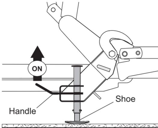
2. Pull and hold lock pin out; then rotate handle UP and release lock pin. It must lock into UPPER hole. Stand hook must grip receiver pin.
