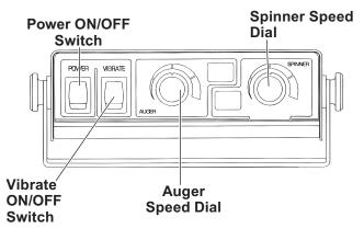
NOTE: The truck ignition must be ON to start the spreader.
