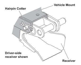
1. Measure the distance "d" from the ground to the top edge of the receiver bracket. Measure both sides and determine average value for "d."
