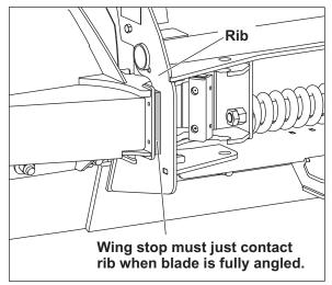
5. Once the stop is making contact with the rib, lock the hex nut into position with the 3/4" jam nut.
