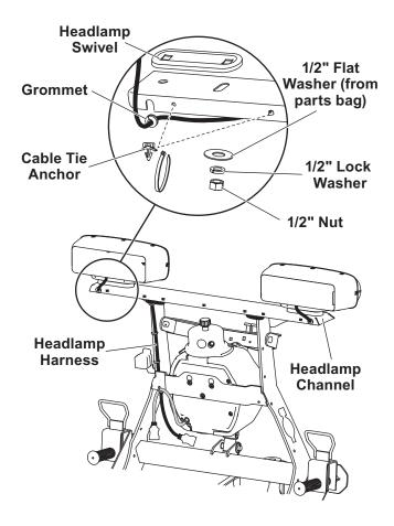
Attach the headlamps and headlamp channel according to the instructions provided in the headlamps box. On the inner headlamp bolt, substitute the 1/2" flat washer from the parts bag for the 1/2" flat washer packed in the headlamps box.
