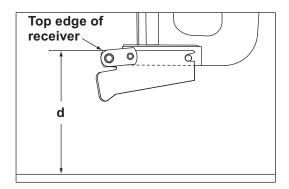
2. Use distance "d" from Step 1 and the following chart to determine the proper pivot plate hole position.
