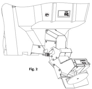
Then rotate the Chute into operating position and lock using two spring latches.
