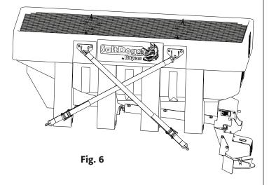
Verify with the vehicle's manufacturer that the factory installed anchor points are designed for tie-down such load. Inspect straps and hardware after each time spreader is loaded. Tighten straps and hardware if necessary.
