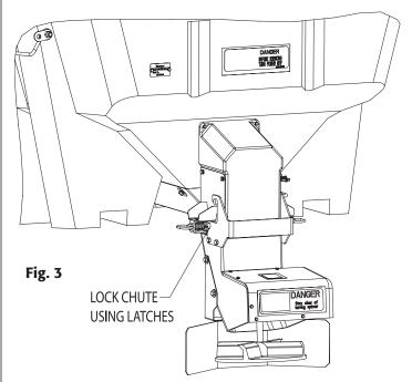
**G.** Slide spreader towards front of the truck leaving adequate space between chute and truck (2-3 inches). Measure the distance from the front of the truck bed to front of the hopper's front legs. Fabricate spacer to fit between front of the spreader and front of the bed per Fig. 4 and Fig. 5
