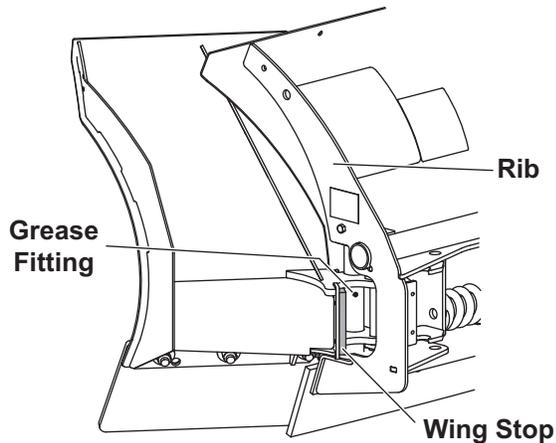
2. If there is a gap between the wing stop and the rib, skip to Step 3.
