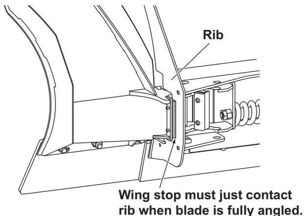
5. Once the stop is making contact with the rib, lock the hex nut into position with the 3/4" jam nut.
