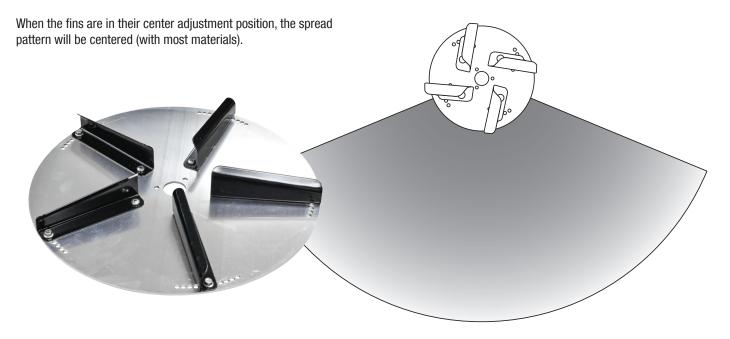
When looking down at the spinner, moving the fins clockwise will adjust the spread pattern toward the left side of the spreader.
