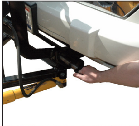
F. Pull handle on drivers side to dis-engage pins then twist until the notch locks open the pins.
