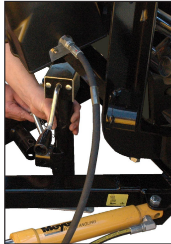
E. Remove crankstand from a-frame.
