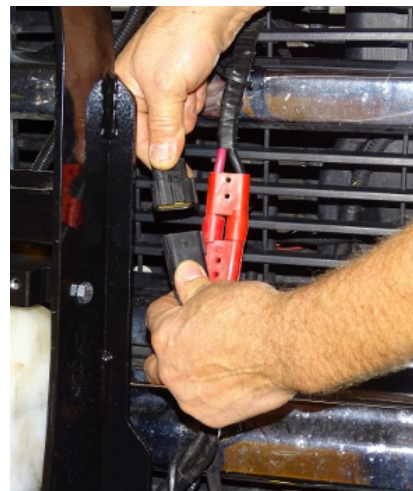
G. Remove weather cover on both ends and connect both electrical plugs.
