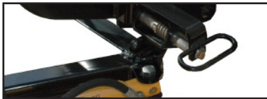
C. Push back on lift frame until pins spring thru mount on vehicle.
