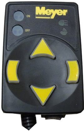
A. Press down button until float light turns blue.
