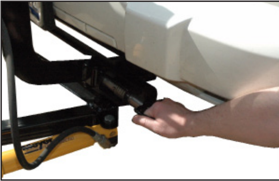
B. Twist handle on driver side to disengage the notch that locks open the pins.
