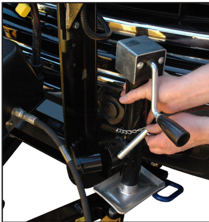
B. Push lift arm down until there is a little slack in the chain.
