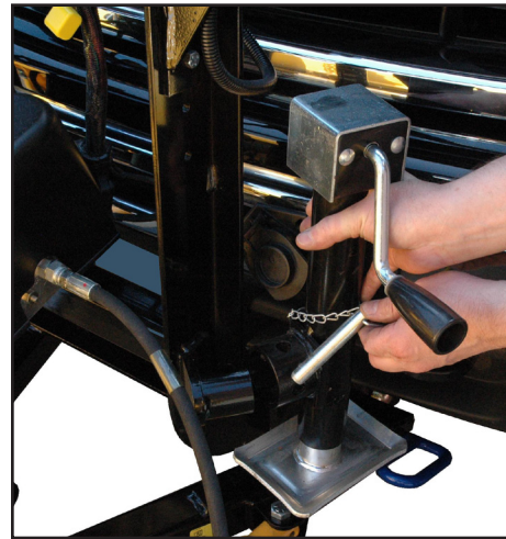
F. Attach crankstand to lift frame.
