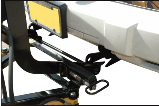
A. Pull vehicle into plow assembly and push plow assembly forward an inch or two.
