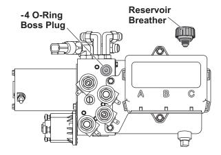
5. Install the pressure switch in place of the O-ring boss plug. Gripping the hex portion only, tighten the pressure switch to 10–13 ft-lb.
